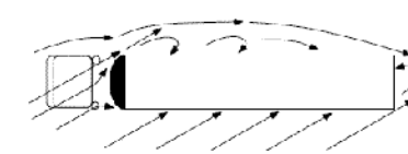
Air striking the NoseCone is smoothly diverted over the top and around the sides of the trailer. Much less turbulence is created, reducing air drag. It also reduces the effect of crosswinds.
